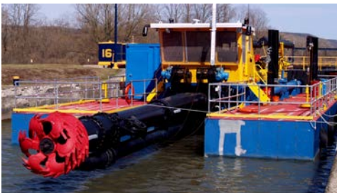
Hydraulic Dredge and Pipeline Disposal. Credit: Ellicott Dredges unit of Baltimore Dredge Enterprises
