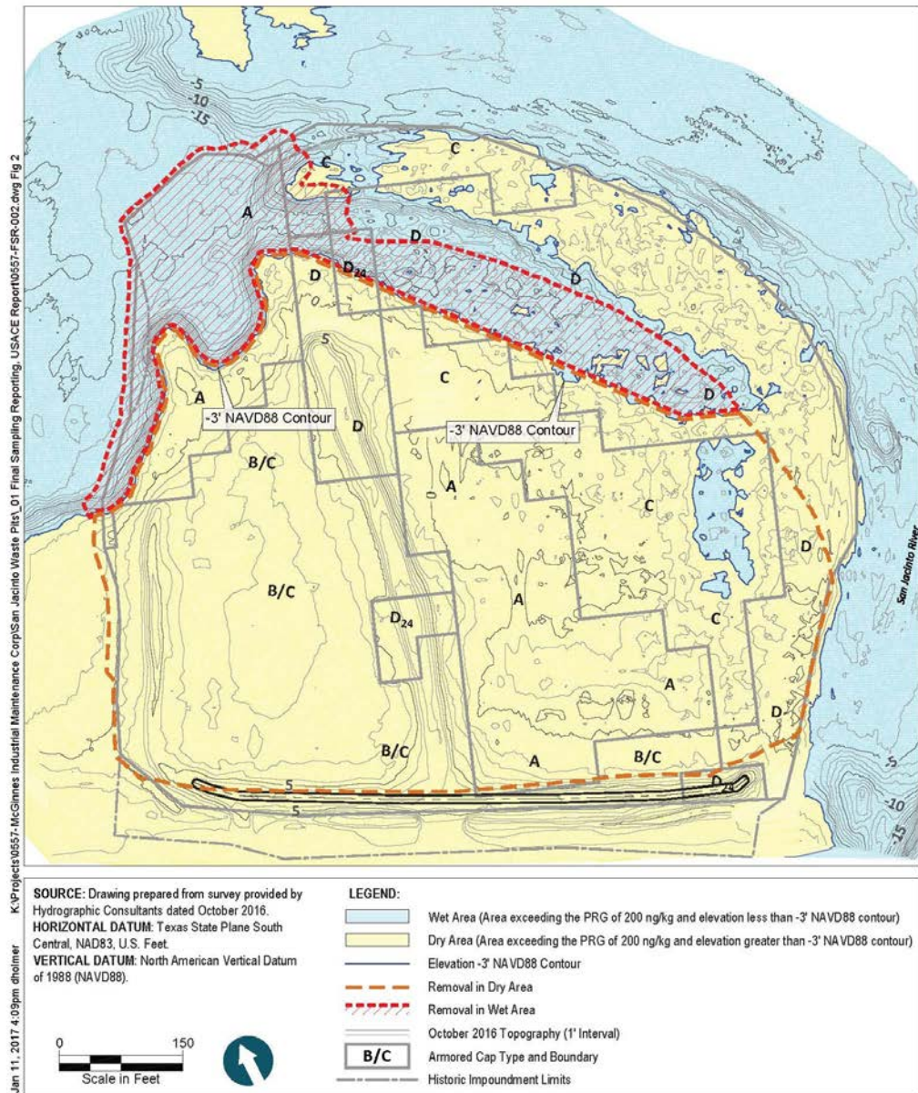
Figure 2. Proposed Plan Removal in the Dry and Wet Areas Using an Approximate -3 Foot NAVD88 Elevation
