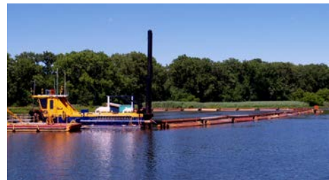
Hydraulic Dredge and Pipeline Disposal. Credit: Ellicott Dredges unit of Baltimore Dredge Enterprises
