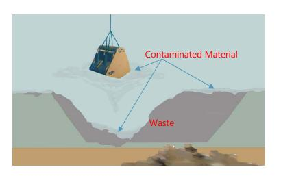
• USACE assumes a new armored cap would be placed over the excavated area to protect remaining contaminated materials from erosion
